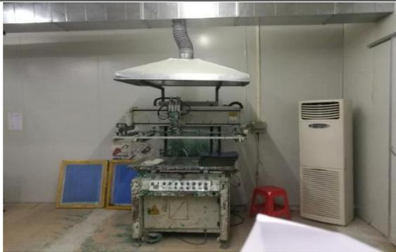
丝印机废气收集罩
